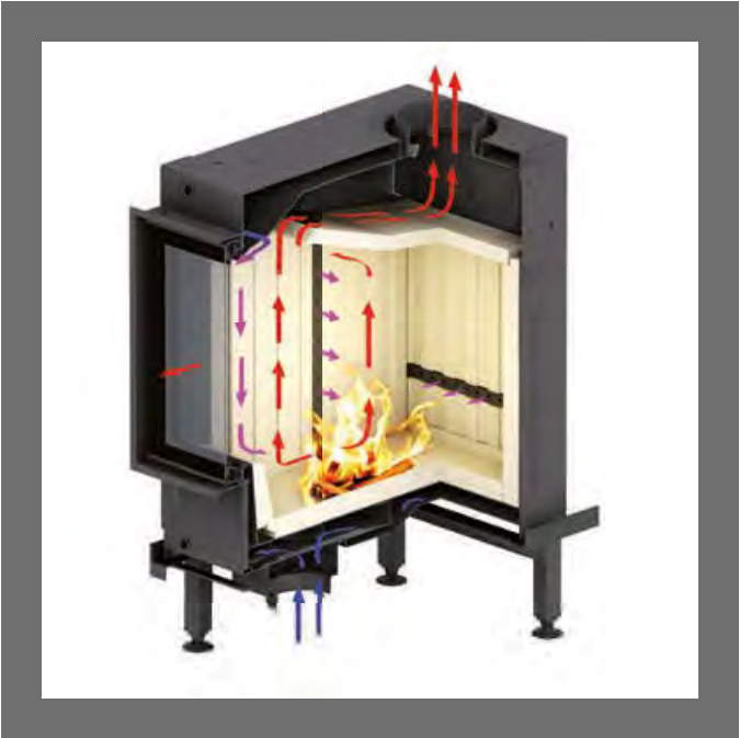
Functional drawing of the Nova F-Air, Classic series heating insert
