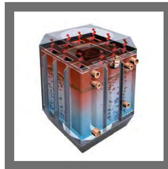
Aquabox with a schematic view of the heat distribution inside the unit
